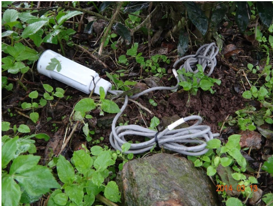
Figure 11. HOBO Pro v2 External Temperature Data Loggers for measuring air temperature and soil temperature.
